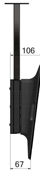
Abmessungen in mm
